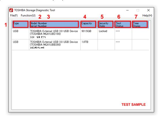
Type : Displays Interface of Drive.Model Number : <External Hard Drive>
