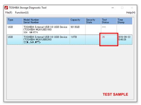
5) During execution of the Zero Filling function, if you would like to stop the Zero Filling function, click "Start/Stop Zero Filling".
